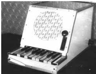
THE THIRD PORTABLE VERSION OF THE RHYTHMICON, BUILT AT THE ACOUSTICAL LABORATORY OF MOSCOW CONSERVATORY. CIRCA 1960.
